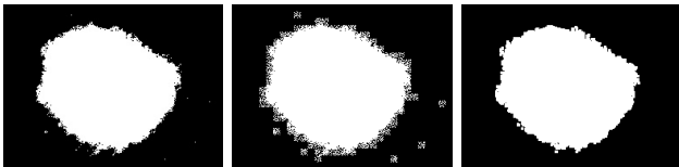
Fig. 6. Left: Original image, Middle: Island Detection, Right: Edge Smoothing and Island removal
